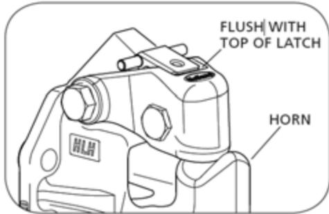
Insert the tethered lock pin through the latch and lock holes, and close the tethered wire lock pin, if applicable (Figure 16).
