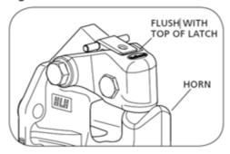
Insert the tethered lock pin through the latch and lock holes, and close the tethered wire lock pin, if applicable (Figure 16).
