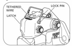
Lift the lock handle away from the vehicle until the lock clears the lock seat on the hook body. Open the latch by rotating the latch assembly up toward the vehicle until the latch is in its most upright position, then release the lock handle. (Figure 17 and 18)
