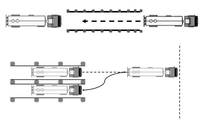
Figure 12.1: Straight Line Backing
