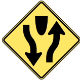
Divided Highway (Road) Begins
